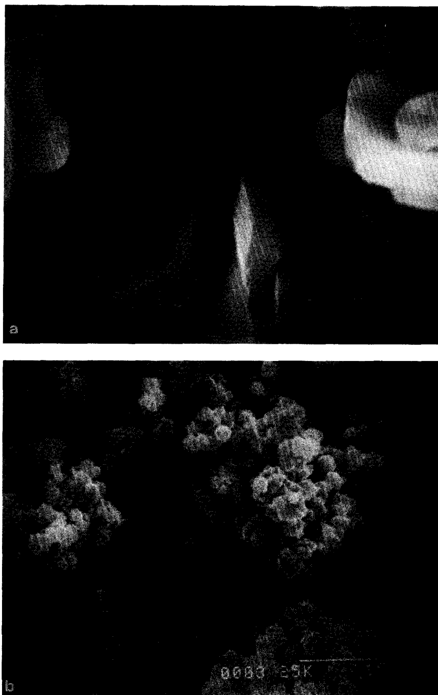
FIG. 4. Scanning electron micrographs of (a) pure \text{MoO}_3 and (b) pure \text{MnMoO}_4 .
